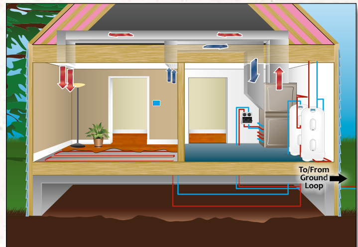
The above illustration depicts a typical combination system installation with forced air and radiant floor in heating mode.
